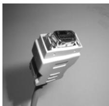
Controller Cable Connector labeled Data
