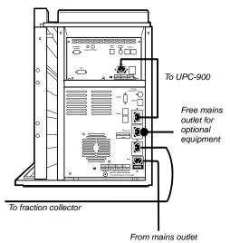
**CAUTION!** The mains power to ÄKTAFPLC must be switched OFF before the UniNet-1 cabling is installed.
