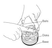
These adapters can also be used as tube racks in the laboratory. The adapter disks are color-coded by the tube size they accommodate; the number of disks used in an adapter assembly depends upon the length of tubes used. Refer to the applicable rotor manual to determine the kind of adapter required for the tubes you are using.
