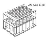
Available sterile or nonsterile 96-cap strips can be used with deepwell plates. (When these caps are used, the capacity of each well is reduced to 1.0 mL.)
