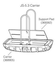
> When using stacked polypropylene plates, place a support pad beneath the bottom plate to prevent breakage during centrifugation. Use the support pad beneath all polystyrene plates.
