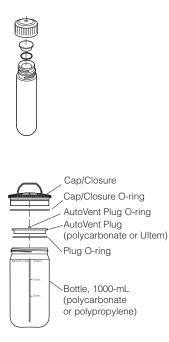
Bottles are available in polycarbonate (hard and clear), polypropylene (translucent), and polyallomer (translucent). Sealed polyallomer or polycarbonate bottles, available for most fixed angle rotors, have a three-piece liquid-tight cap assembly. Other bottles have screw-on caps. Cap assemblies should always be removed before autoclaving bottles. Bottle selection depends on the rotor in use and the specific application; refer to the applicable rotor manual.
