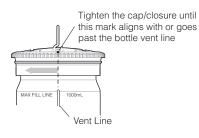
Place the plug on the bottle, then screw on the cap/closure by hand as tightly as possible. Tighten until the timing mark on the cap/closure is aligned with or goes past the vent line on the bottle.
