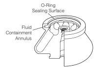
A feature of many Beckman Coulter fixed angle rotors is a patented fluid-containment annulus, located below the O-ring sealing surface. If tubes are overfilled or if leakage occurs during centrifugation, the annulus holds enough volume that all of the liquid is kept inside the rotor—even if all tubes leak at the same time. This feature virtually eliminates the escape of liquid into the centrifuge chamber.
