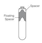
Quick-Seal tubes require spacers made of anodized aluminum, with or without floating spacers. The particular combination depends on the type of rotor being used and the tube size.
