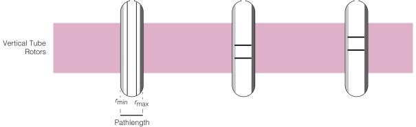
Figure 1-2. Particle Separation in Fixed Angle, Swinging Bucket, and Vertical Tube Rotors. Dark gray represents pelleted material, light gray is floating components, and bands are indicated by black lines.
