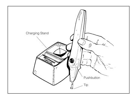
Figure 3-1. The Cordless Quick-Seal Tube Topper
