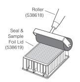
Seal & Sample aluminum foil lids (538619) have a bioinert adhesive backing, enabling complete plate sealing. The lids are presized for multiwell, deep-well, and square-well plates, and cause no reduction in well capacity. A 4-inch soft-rubber roller (538618) is required to ensure secure sealing of the foil lids.
