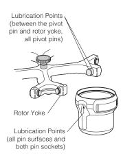
*JS-4.2, JS-4.2A, and JS-4.2SMA Rotors* — Approximately every three months (or every 250 runs), and after cleaning and/or autoclaving the rotor, lubricate the contact areas between the buckets and the pivot pins.
