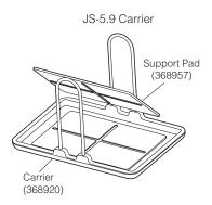
High-impact thermoplastic carriers are used in the JS-5.9 and JS-5.3 rotor buckets to provide support to labware during centrifugation and facilitate loading and unloading buckets. Each rotor bucket can carry a 96-well kit for high-throughput processing (such as a DNA or RNA kit), or standard microplates used in the serial dilution of small liquid volumes—up to five (JS-5.9) or six (JS-5.3) stacked 96-well polypropylene plates, two (stacked) deep-well plates, or one square-well plate per bucket.
