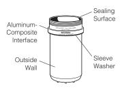
Some J series rotors have attached windshields to reduce air friction. The windshields are made of anodized aluminum.
