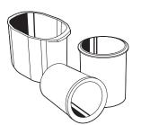
Polypropylene blood bag cups are available for use in swinging bucket rotors to obtain cell-free plasma for cell packing or for leukolyte depletion. Different sizes of cups are available to accommodate single, double, triple, or quad pack blood bags. Refer to the applicable rotor manual to determine the correct blood bag cup to use. Blood bag cups are autoclavable.
