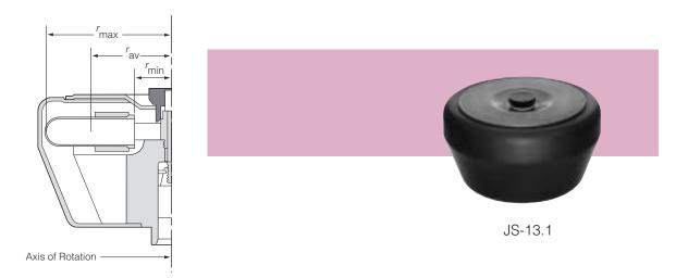
Figure 5-1. Examples of Swinging Bucket Rotors
