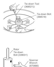
• JS-4.2A and JS-4.2SMA—secure the rotor to the drive hub with the tie-down bolt (368518). Tighten the bolt with the tie-down tool (368521), then remove the tool.
