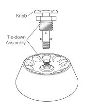
To secure the rotor to the drive spindle hub during centrifugation, J series rotors are equipped with devices that screw into the hub. If the rotor is left in the centrifuge between runs, tighten the tie-down device before each run.
