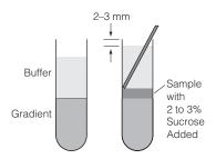
For *thinwall* tubes only partially filled with gradient, add a buffer solution to fill the tube to provide tube wall support. Although the gradient volume is reduced, sample volume is not changed.
