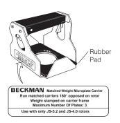
Carriers used with the JS-5.2 and JS-4.0 rotors are NOT interchangeable with those used with the JS-4.2, JS-4.2A, JS-4.2SM, JS-3.0, and JS-2.9 rotors. If you have more than one type of carrier, check the label on the side of the carrier to make sure that you are using the right one for your rotor. Table 5-2 lists carriers used with J6 rotors.
