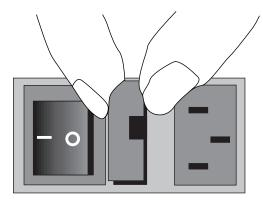
Figure 4.2: Removing the Fuse Box
