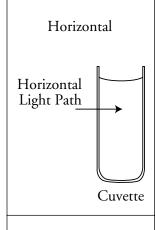
The standard pathlength of a cuvette is the conventional basis for quantifying the unique absorptivity properties of compounds in solution. Quantitative analyses can be performed on the basis of extinction coefficients, without standard curves (e.g., protein at 280 nm, nucleic acid estimates at 260 nm and NADH-based enzyme assays). When using a cuvette, the pathlength is known and is **independent** of sample volume, so absorbance is proportional to concentration.
