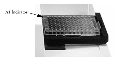
Figure 1.4: Microplate Drawer
