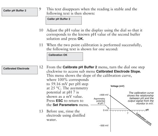
A new electrode typically has a slope of 95 - 102% and an asymmetry potential within  $\pm 30$  mV. As the electrode ages, the slope decreases and the asymmetry potential increases.
