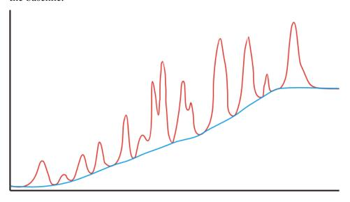
Example of a UV curve after subtraction of the baseline
