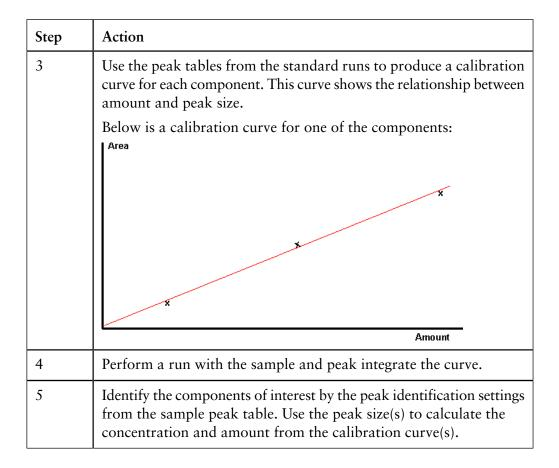
Illustration - how to use the calibration curve The illustration below describes how the calibration curve is used to determine the amount based on the sample peak area.
